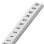
Zack Marker strip, flat, Strip, white, labeled, printed horizontally: consecutive even numbers 2 ... 20, 22 ... 40, etc. up to 82 ... 100, mounting type: snap into flat marker groove, for terminal block width: 5 mm, lettering field size: 5.15 x 5.15 mm, Number of individual labels: 10
