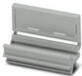
Group marking label, snaps onto terminal center for screw, spring-cage and quick connection terminal blocks, labeled with ESL 26x6 mm or EST 25x6 mm, in the foot part with Zack marker strip, length: 29 mm
