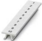
Zack marker strip, white, Printed vertically: consecutive numbers 1 ... 10, 11 ... 20, etc. up to 491 ... 500, mounting type: snap into tall marker groove, for terminal block width: 5.2 mm, lettering field size: 5.15 x 10.5 mm
