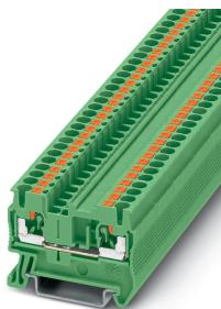
Feed-through terminal block, nom. voltage: 800 V, nominal current: 24 A, connection method: Push-in connection, 1 level, Rated cross section: 2.5 mm<sup>2</sup>, cross section: 0.14 mm<sup>2</sup> - 4 mm<sup>2</sup>, mounting type: NS 35/7,5, NS 35/15, color: green
